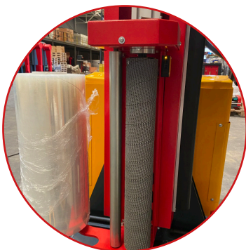
Contact safety system in the wrapping arm
