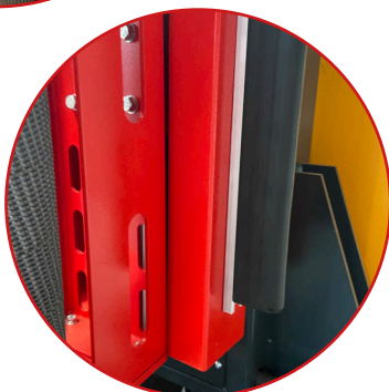
Contact safety system in the wrapping arm
